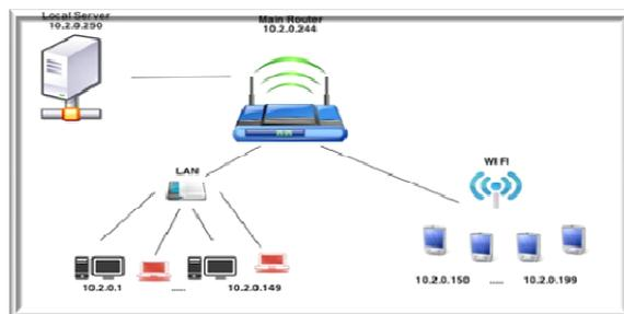
FIGURE 1 NETWORK SCHEME IN AN IPV4 PROTOCOL LAYOUT
